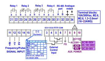
Please check the voltage of power supplied first, and then connect to the specified terminals. It is recommended that power supplied to the meter be protected by a fuse or circuit breaker.
